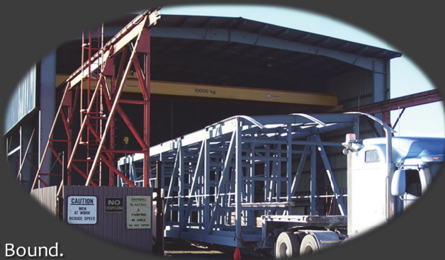
* Above, a 35 ft. crane clearance enables our shop to fabricate a 30 ton truss.
